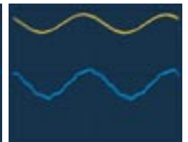
Current waveform at the frequency inverter with harmonic filter type HFM-FB
